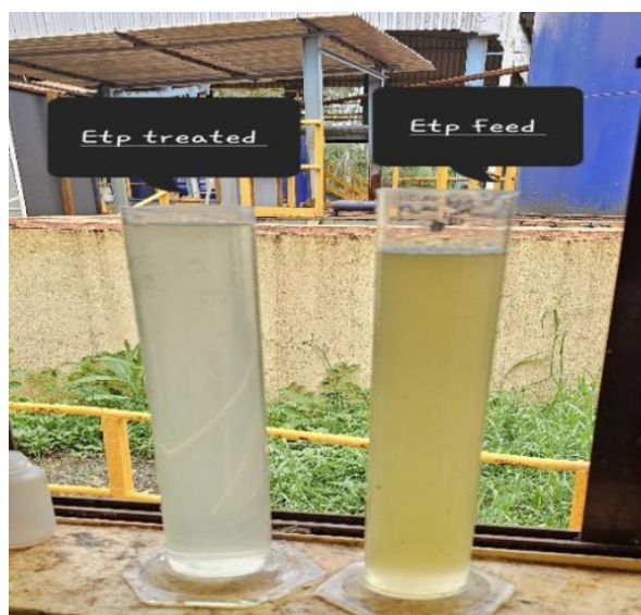
Figure 2. Jar test with ETP feed and treated water.
